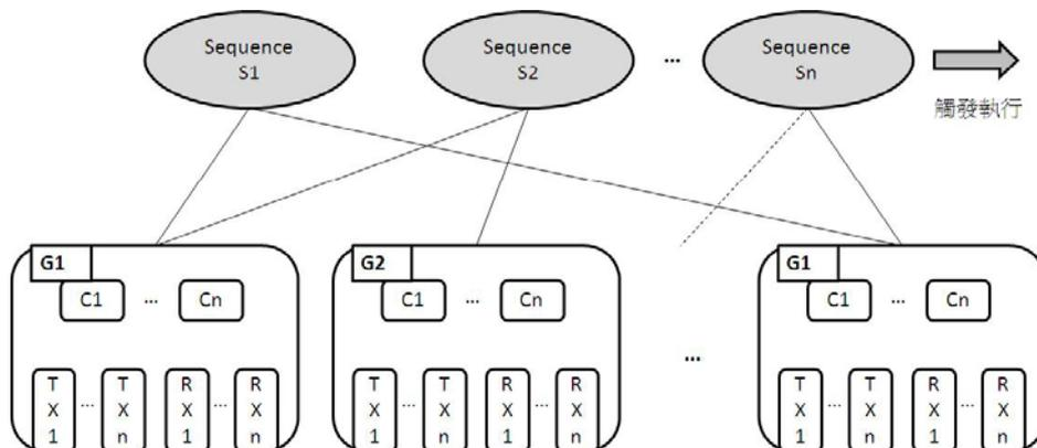
First of all, establish the transmission instructions (TXs) and the reception instructions (RXs) in the group. Then, set the execution sequence and the number of times for TXs and RXs through the commands.
