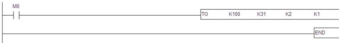
After M0 is triggered, COM1 on SCM module will keep reading the present value which will be stored in D100, and the status value of bit0 in D100 is 1.
