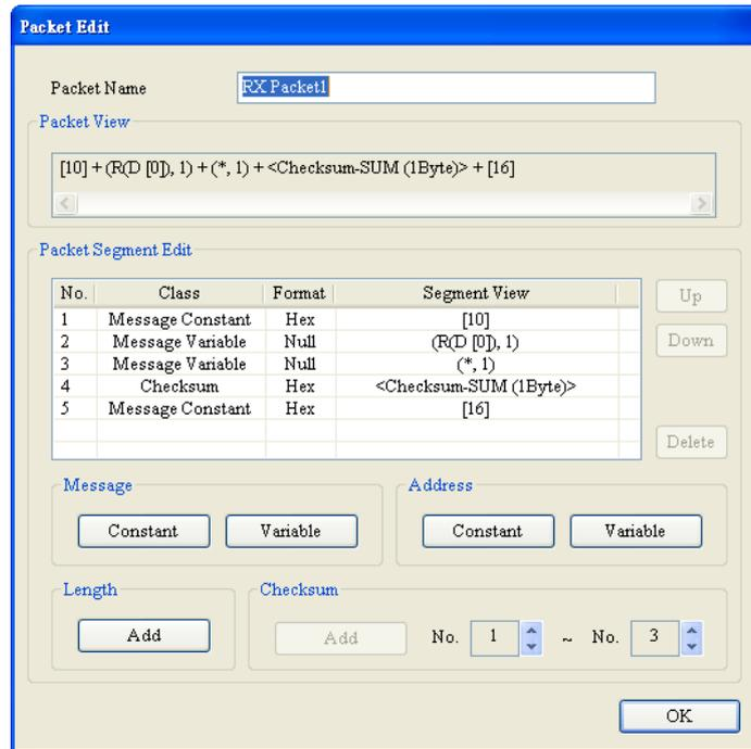
Edit the command: Sending Tx Packet1, and receiving Rx Packet1
