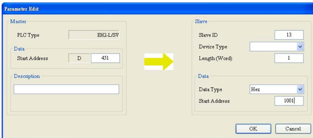
After the setting is complete, the user can designate the communication port used in Modbus Advance – COM port 2 on left-side module number 1.
