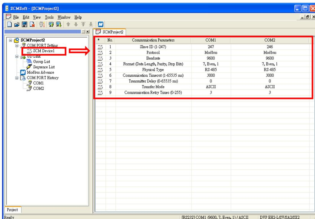
Set the communication parameters of COM1: station number 247 (default), Modbus RTU, 9600, 8, Even, 1.
