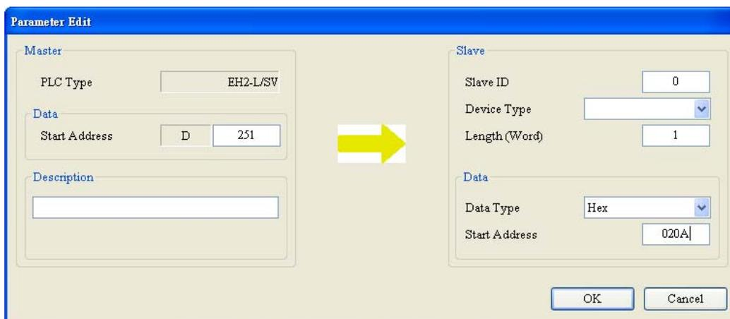
PLC (master D300~D309←slave D100~D109), (master D350~D354→slave D150~D154)
