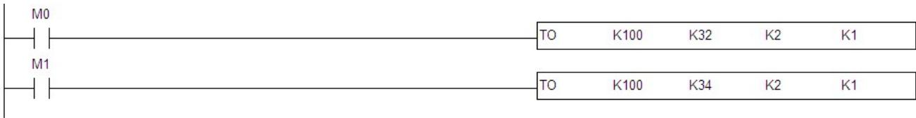
After M0 is triggered, the data will be read from the slave address which has been set through COM2 on SCM module.
